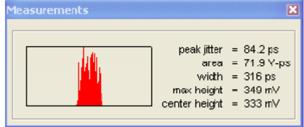
6 meter 28-awg unequalized assembly with 4 near end aggressors on one side QAAAA
